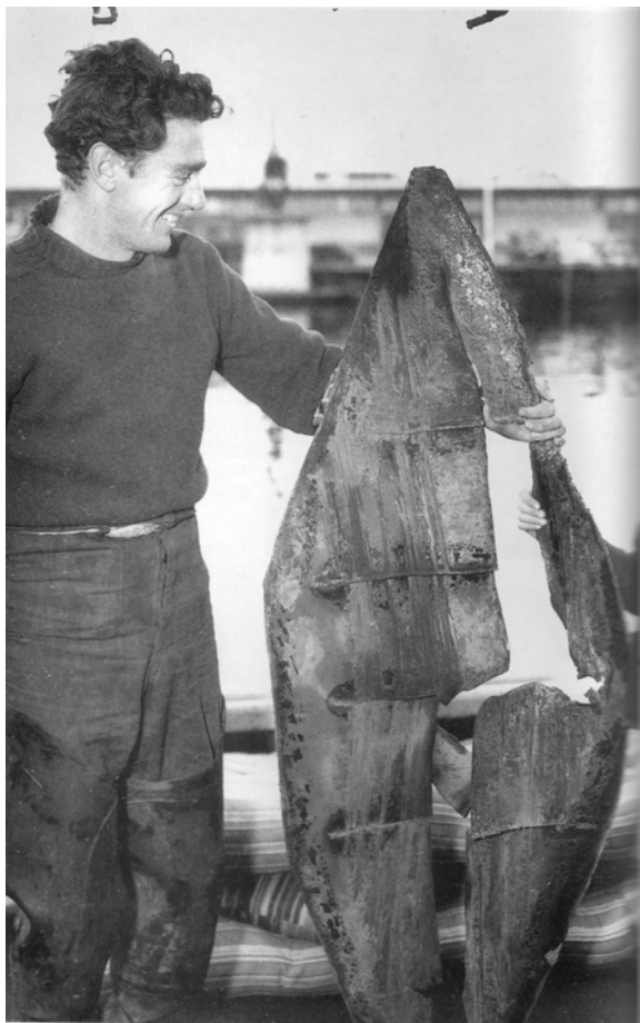
Crewman Ron 'Crash' Howells with a section of Patanela's damaged bow after hitting an uncharted rock in north-west Tasmanian waters. Constitution Dock, Hobart, 1958.
